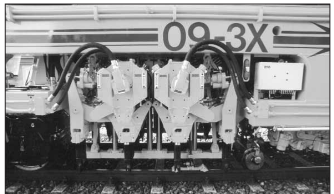
Fig. 6: Three-sleeper tamping unit of the continuous three-sleeper tamping machine 09-3X Tamping Express
