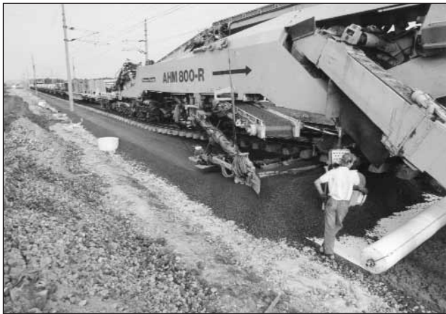
Fig. 10: AHM 800-R formation rehabilitation machine
