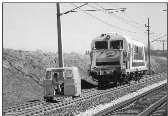
Fig. 9: EM-SAT 120 track survey car
