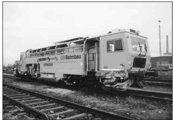
Fig. 8: UNIMAT Sprinter spot fault elimination machine
