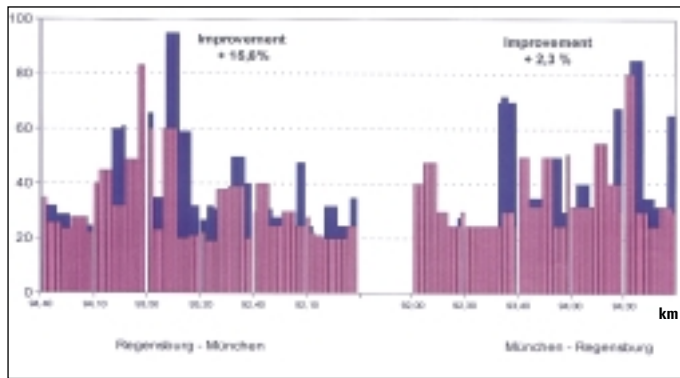
Fig 5. Comparison of track geometry on unstabilised test sections measured using DB's SR disturbance analysis method before maintenance (blue) and after one year of traffic (pink)
